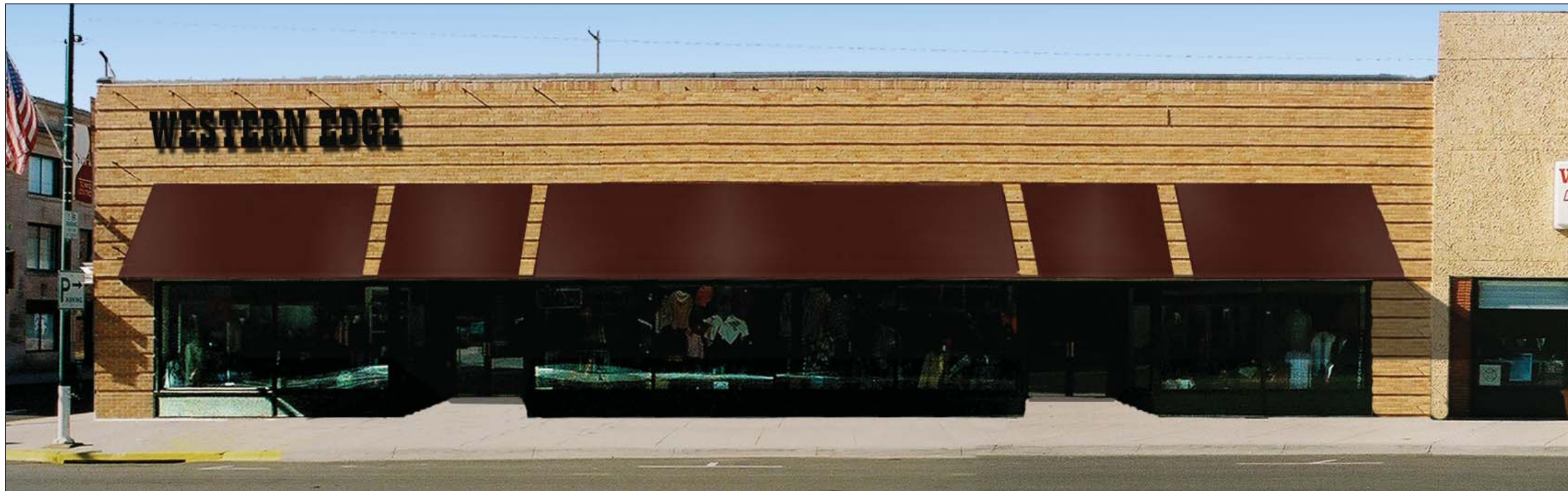
Image 6. Option 3. Awnings fabricated with Sunbrella's Mahogany (#4667) fabric articulate the store entrances and provide shading for the display windows, as well as weather protection for pedestrians. The signage, in "Billboard 11 Wide" font, is mounted to align with the awning at the corner of the building.
