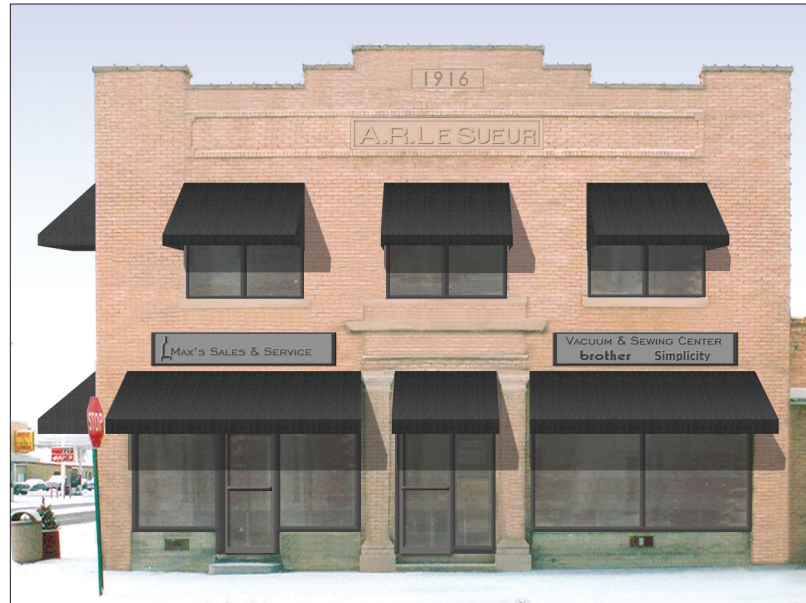
Image 12. Option 4 (east). The same changes as in Options 1 through 3 are made here, except the window frames are painted dark brown. Awnings in Sunbrella "True Brown" (#4621) are added. Sign boards, with dark brown and light brown paint, are attached to the building on either side of the main entrance.
