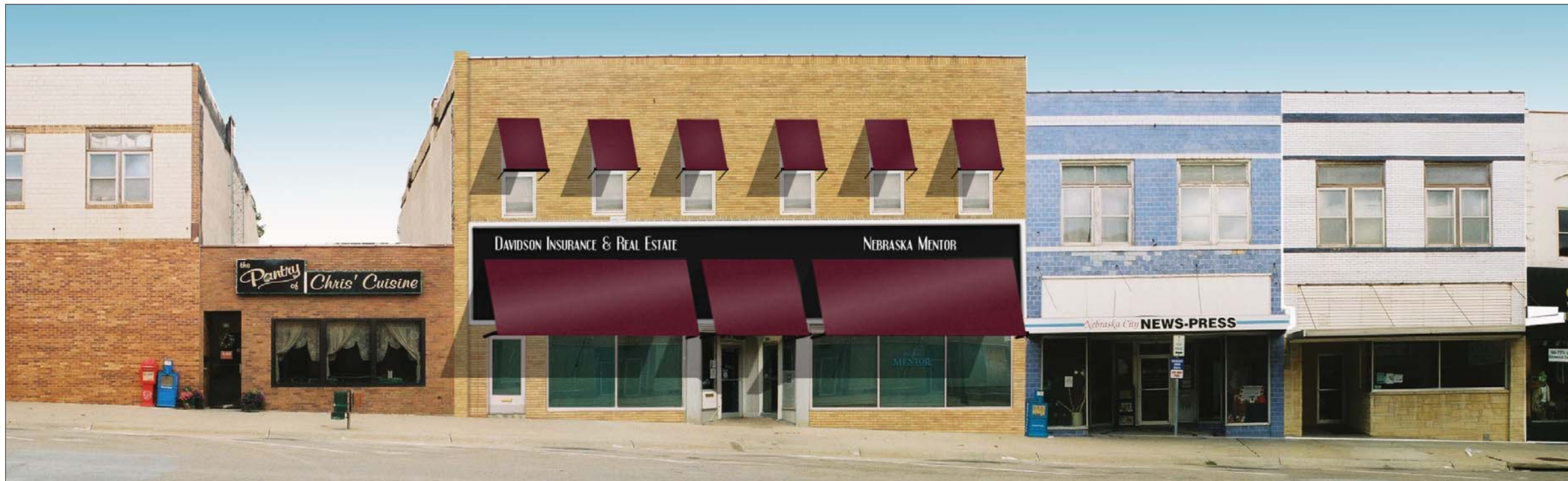
Image 4. Option 1. The existing large signboard is resurfaced with an alternative material, such as an exterior insulation and finish system (EIFS)—a plasticized stucco coating over foam board insulation. Awnings fabricated with Sunbrella's "Burgundy" (#4631) fabric articulate the two storefronts and the shared recessed entryway. The signage ("Engbrechtre" font), identifying the two tenants in the first floor spaces, is centered above each of the two storefront awnings. The second story windows are shaded by individual awnings.
