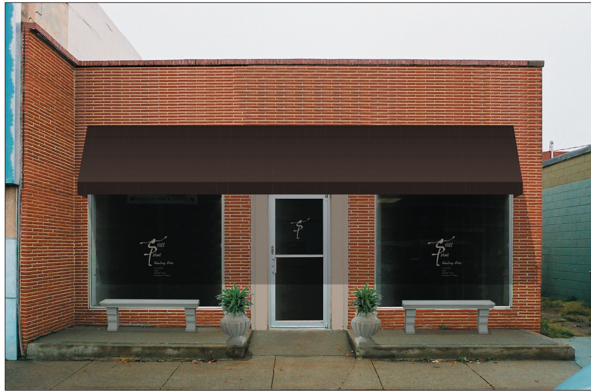
Image 13: Option 10. One continuous awning in Sunbrella fabric Walnut Brown Tweed (4618) is centered on the facade. The signage is applied to the front windows and top of the door glass. Two concrete benches and two concrete planters are placed on the concrete platforms that flank the door.
