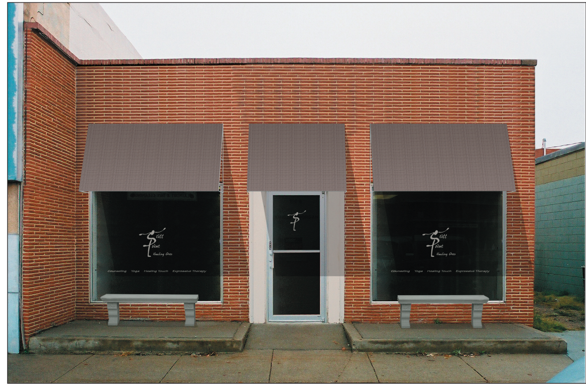
Image 10: Option 8. Three separate awnings in Sunbrella fabric Linen Tweed (4654) are centered above the windows and door. As with Option 4, these awnings have no sides or valances. Still Point logos are applied to the windows and front door glass. Concrete benches flank the front door.
