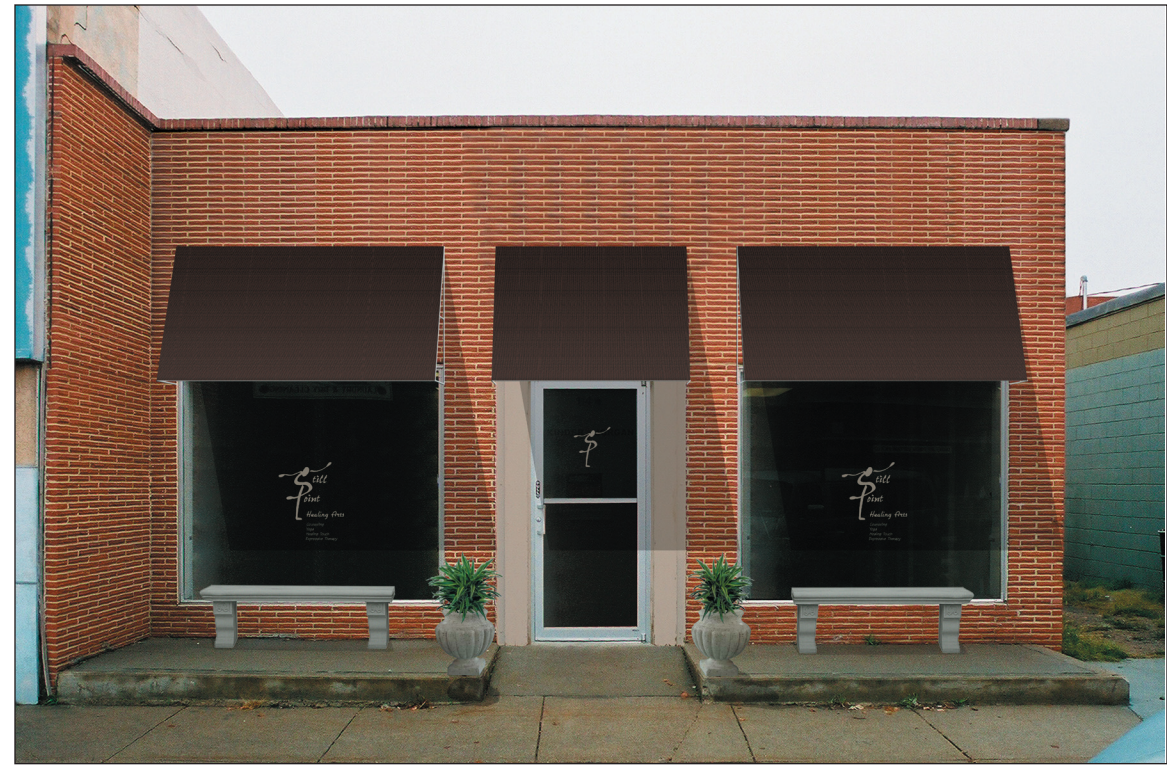
Image 14: Option 11. Three separate awnings in Sunbrella fabric Walnut Brown Tweed (4618) are centered above the windows and door. As seen in Options 6 through 8, these awnings are simply sloping planes without sides or valances. Still Point logos are applied to the front windows and door. Concrete benches and planters flank the entrance.
