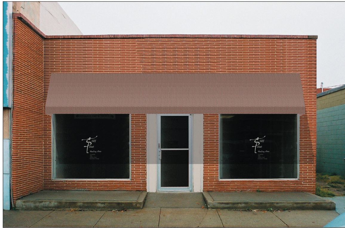
Image 5: Option 4. The metal siding is removed from the facade in Options 1 through 9. One continuous awning in Sunbrella fabric Mocha (4616) is centered across the facade. Business logos are applied to both front windows.
