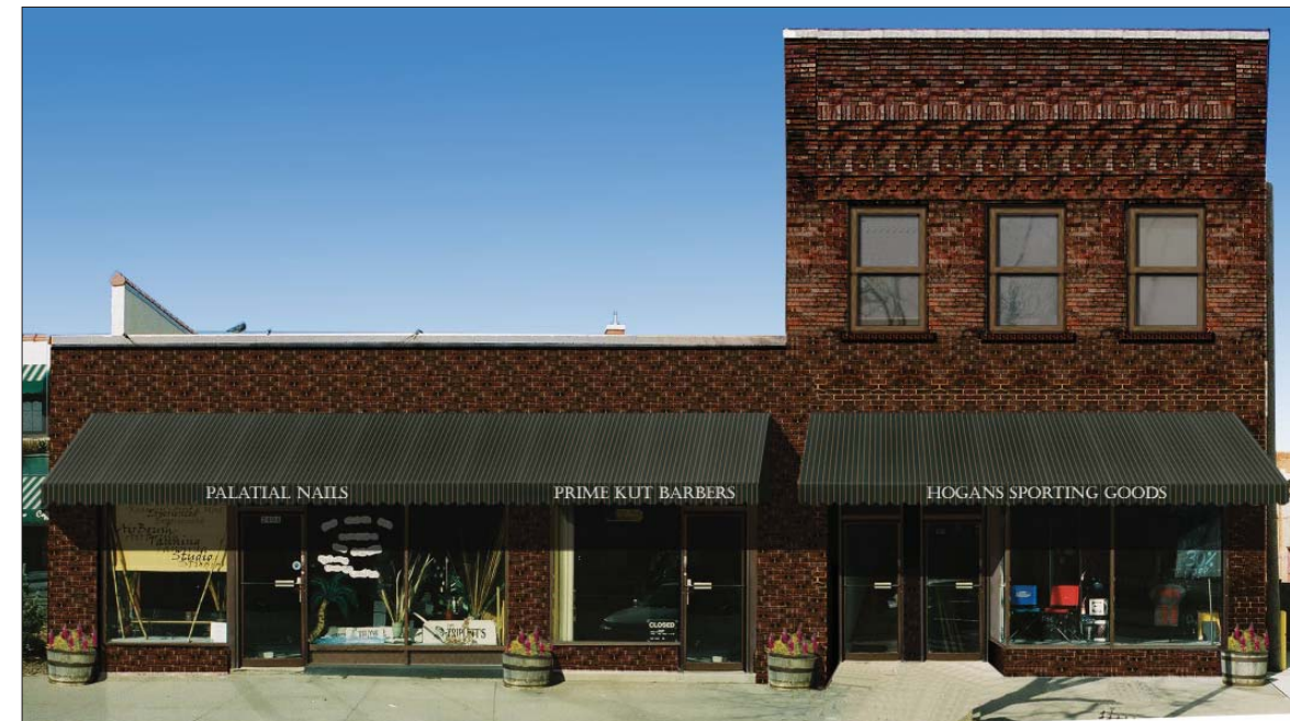
Image 13. Option 3.3: Two conventional fixed awnings are installed on the storefronts, one on the one-story portion of the building, and one on the two-story portion of the building.
