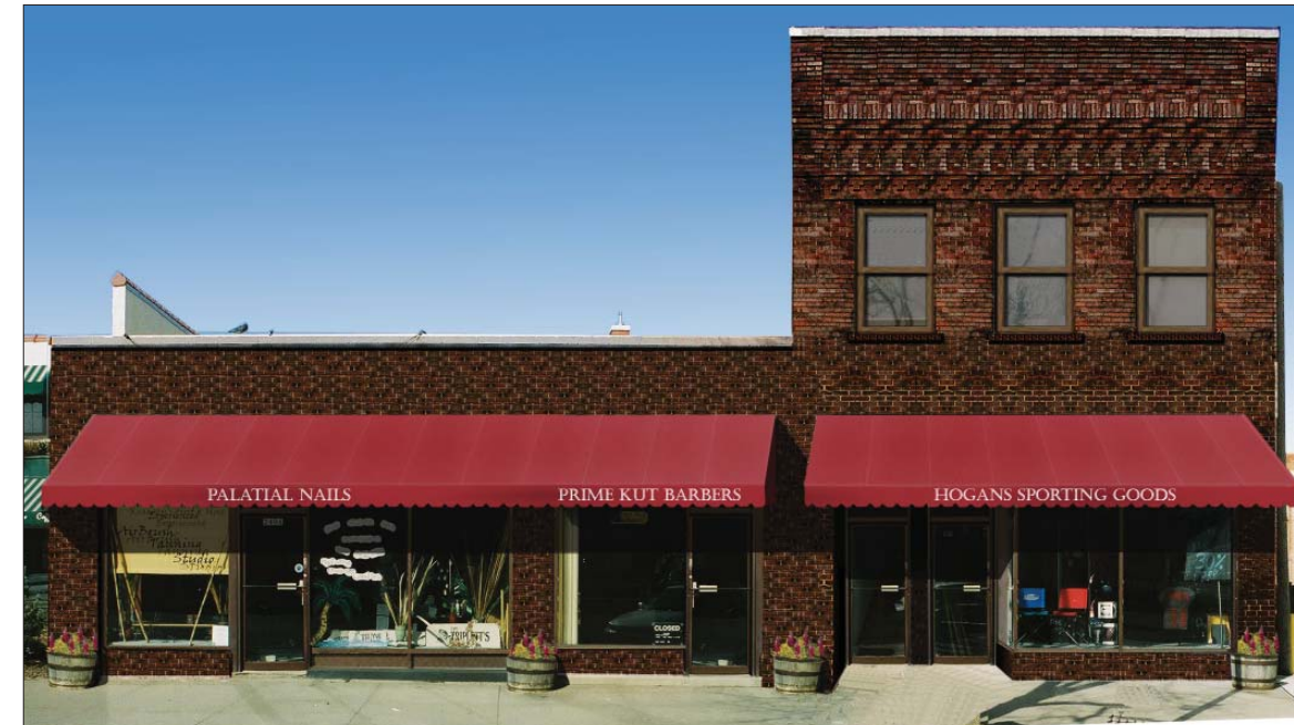
Image 7. Option 1.3: Two conventional fixed awnings are installed on the storefronts, one on the one-story portion of the building, and one on the two-story portion of the building.
