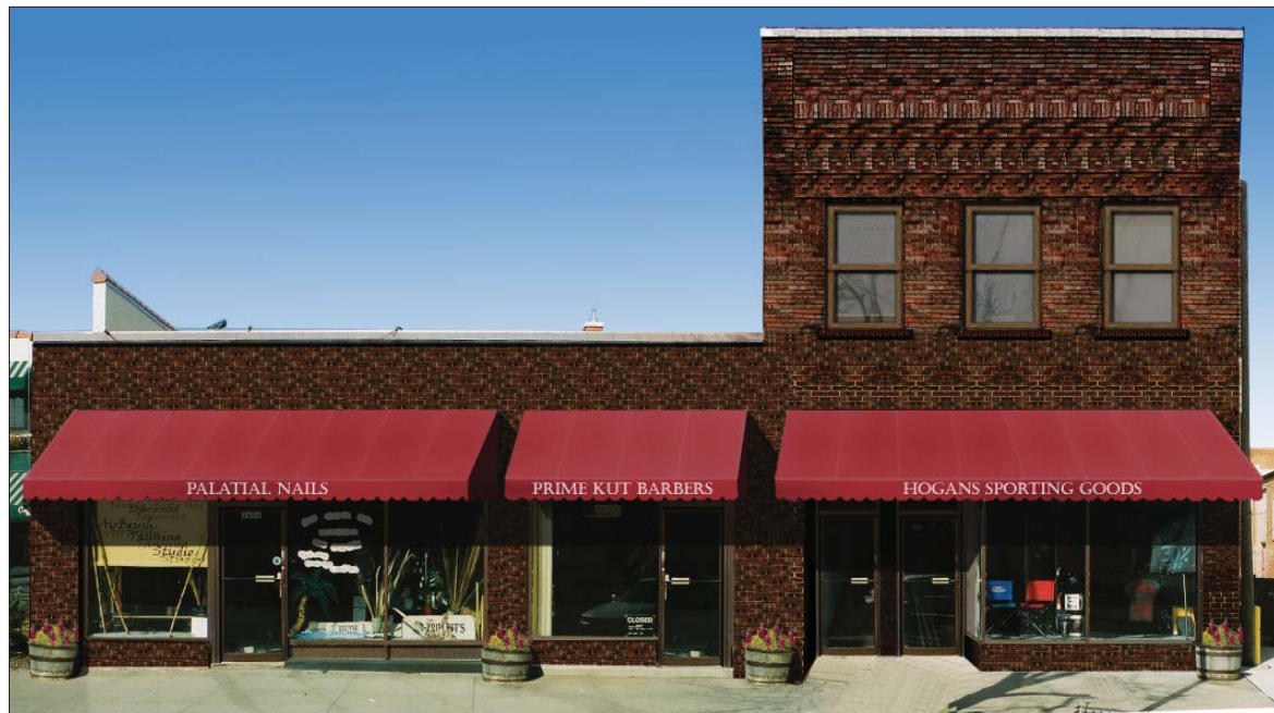
Image 6. Option 1.2: Three conventional fixed awnings are installed on the storefronts to demarcate the three stores in the building.
