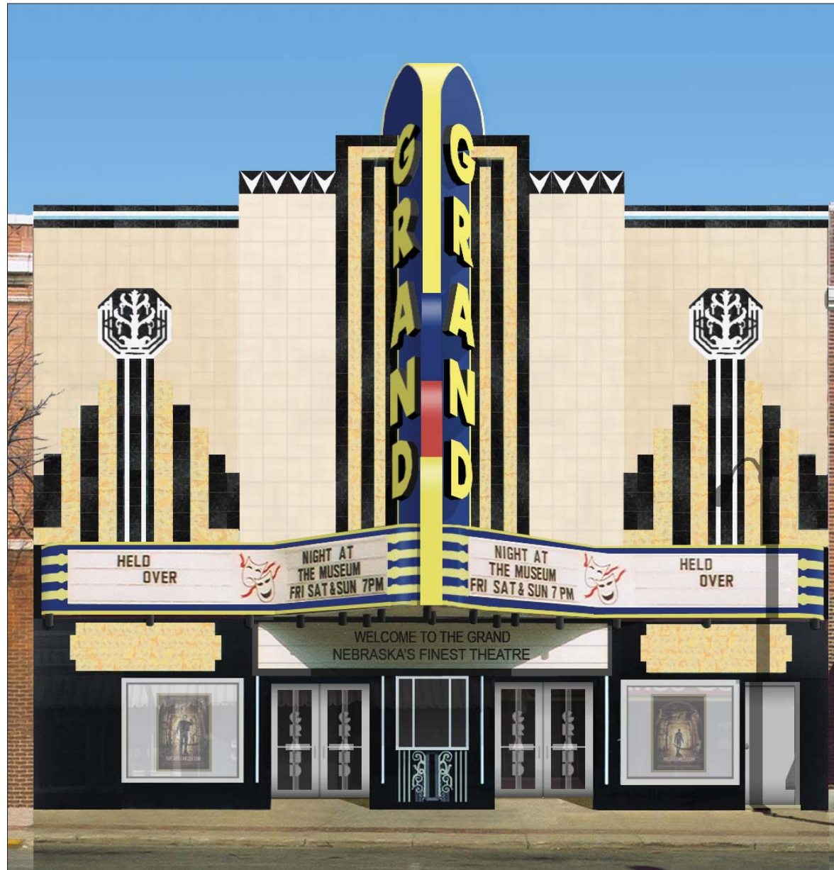
Image 16. Alternative Scheme using Fiordo Tile (Option 4): Fiordo's "Sand Levigato" 8" x 16" porcelain tiles are used on the upper facade, as described in Image 8 and Table 2 "Upper Facade". The paint scheme of the signage is representative of the colors and design depicted in Image 3.
