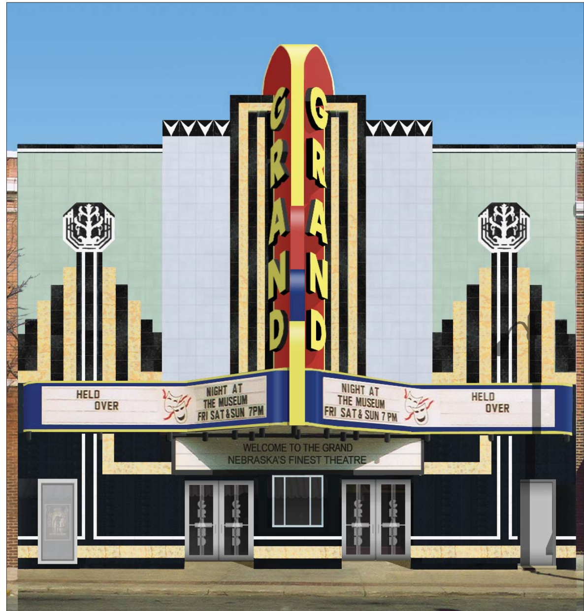
Image 15. Alternative Lower-Facade (Option 3): This image depicts a second alternative for the lower-facade. Again, the tile design is meant to help connect the lower-facade to the upper-facade. As in Image 14, a display window has been installed. The "GRAND" signage uses a different color scheme.
