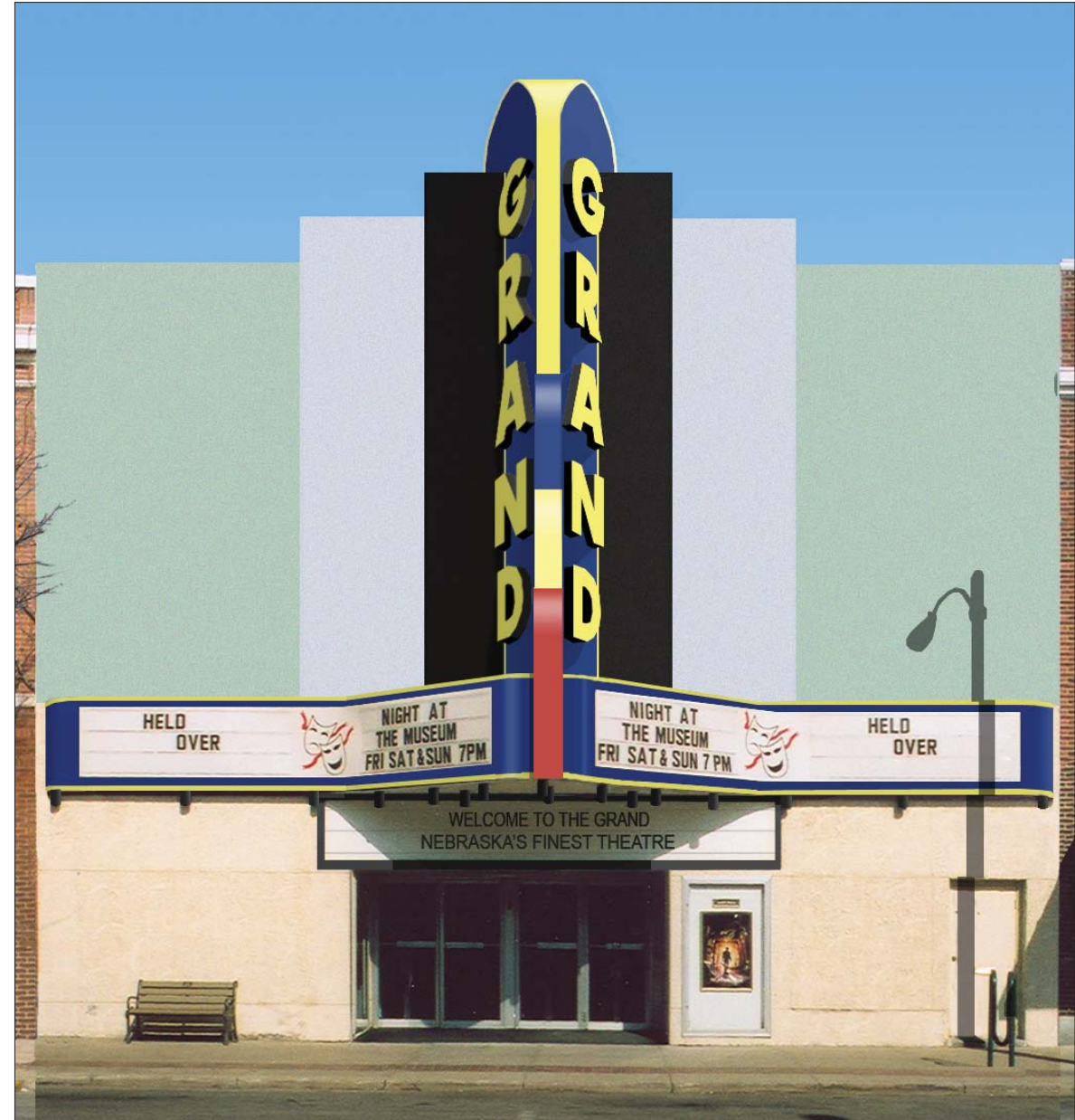
Image 10. Stage Two Restoration: For the second stage of the process, the stucco on the upper-facade has been painted in a pattern reminiscent of the glass tile-work to be restored.
