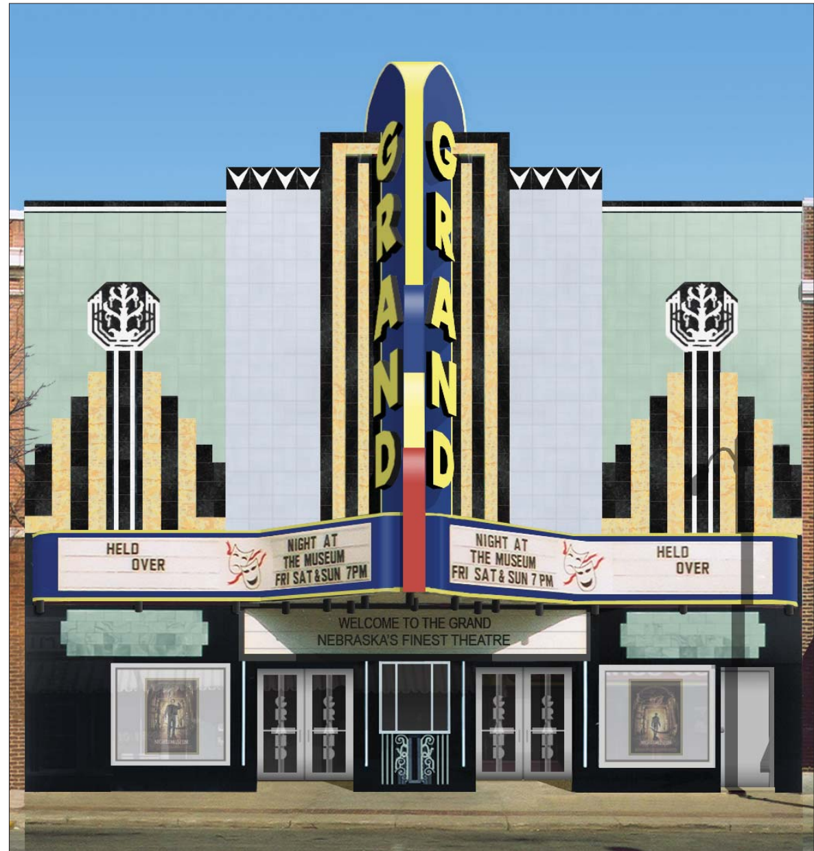
Image 12. Stage Four Restoration (Option 1): The final stage of restoration would remove the stucco from the upper-facade to be replaced with glass tiles, as depicted in Image 8 and Table 1. The coloration of the facade is taken from historical photographs and common Art Deco theatre coloration schemes.
