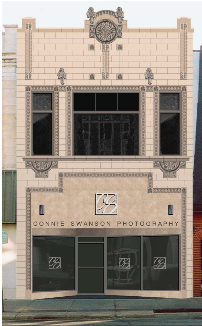
Image 18: Option 2. The former transom window and signboard opening has been replaced with porcelain tile, a sample of which is depicted in Image 17. The signage is black flat cut metal in Arial font available from Gemini ( http://www.signletters.com ). The custom logo would be made using flat cut metal.
