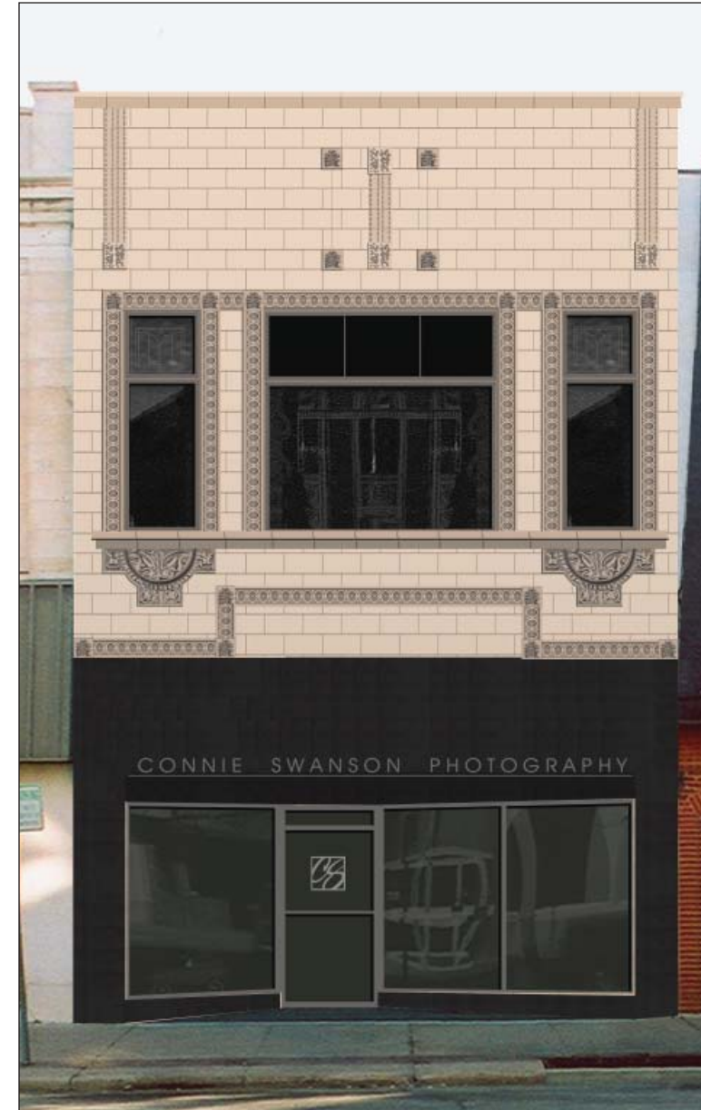
Image 23: Option 3. This proposal replaces damaged or lost terra-cotta units on the lower portion of the building with porcelain tile, a sample of which is depicted in Image 24. The signage is flat cut metal in Times Roman font available from Gemini ( http://www.signletters.com ).
