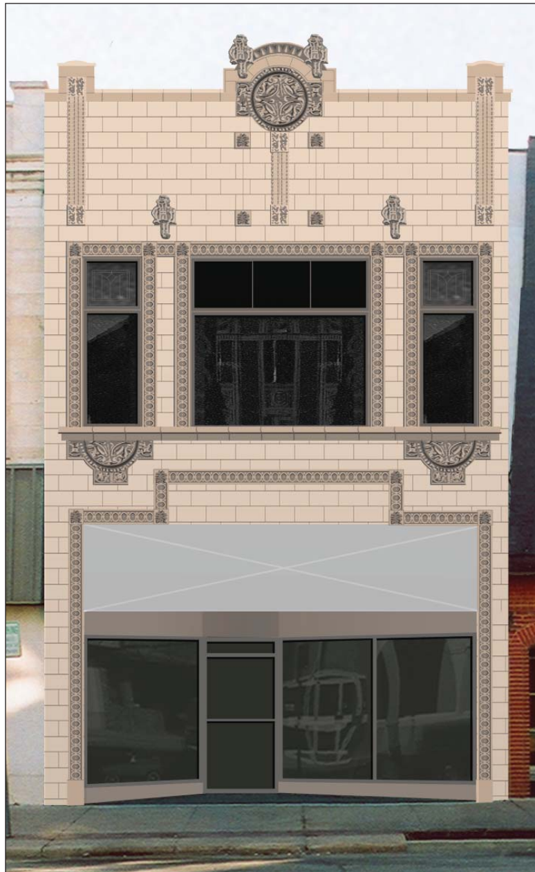
Image 10: Fully Restored Terra-cotta. This view shows the building if the terra-cotta is fully restored. The original cornice has been reproduced and replaced.
