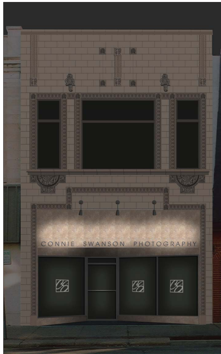
Image 22: Option 3. This proposal suggests flat cut metal in Avant Garde Medium font available from Gemini ( http://www.signletters.com ) for the signage. SPJ Lighting's Aluminum Sign Lights (SPJ51-05) are used to illuminate the signage.
