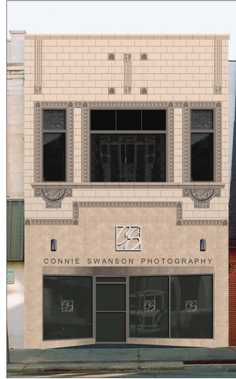
Image 20: Option 2. Otherwise similar to Images 18 and 19, this proposal replaces damaged or lost terra-cotta units on the lower portion of the building with porcelain tile, a sample of which is depicted in Image 17.
