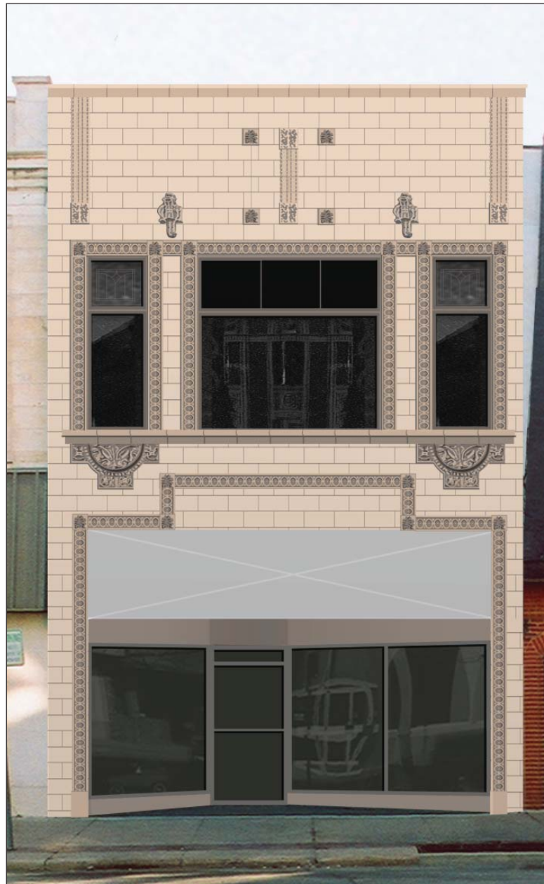
Image 11: Partially Restored Terra-cotta. This view shows the building if the terra-cotta is partially restored. A simplified cornice has been added, while the remainder of the building is restored by replacement of damaged terra-cotta units with reproduction units.
