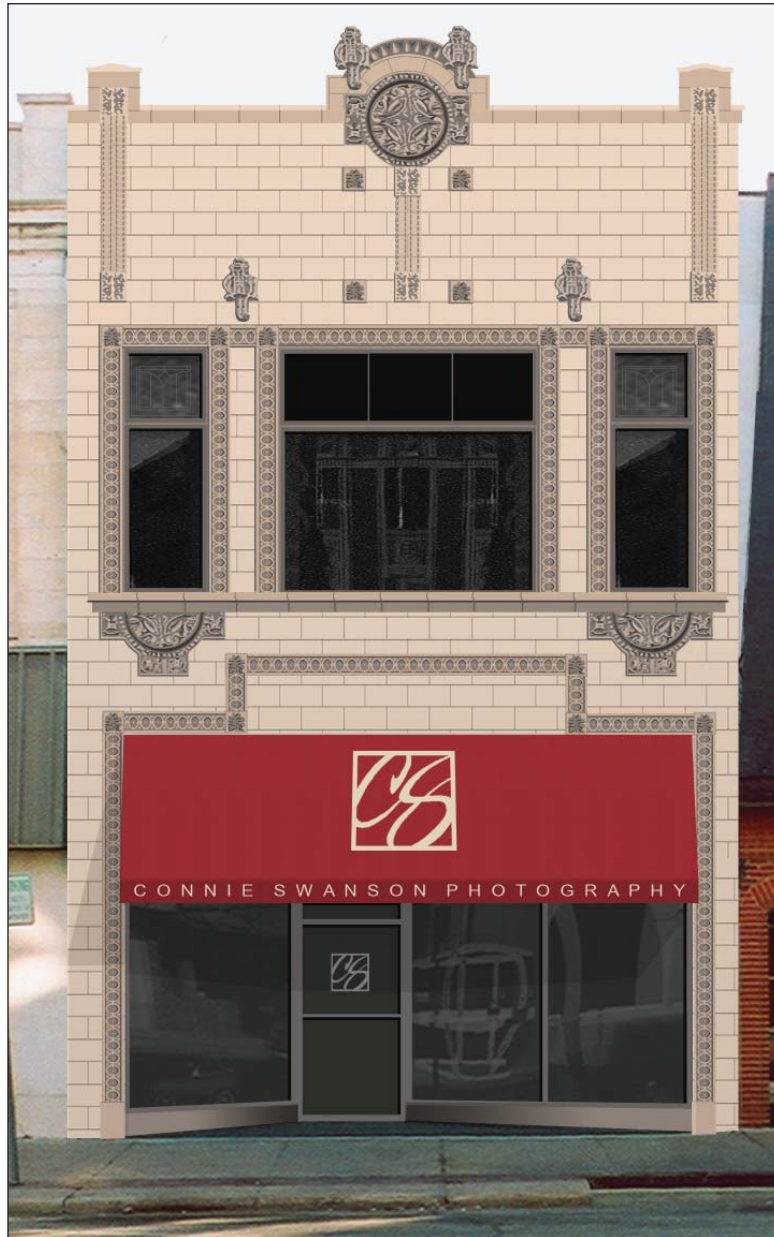
Image 25: Option 4. The former transom window and signboard opening has been covered with an awning fabricated with Sunbrella's "Logo Red" (style 4666) fabric, a sample of which is depicted in image 28. Signage has been applied with graphic film directly onto the awning fabric with Arial font.
