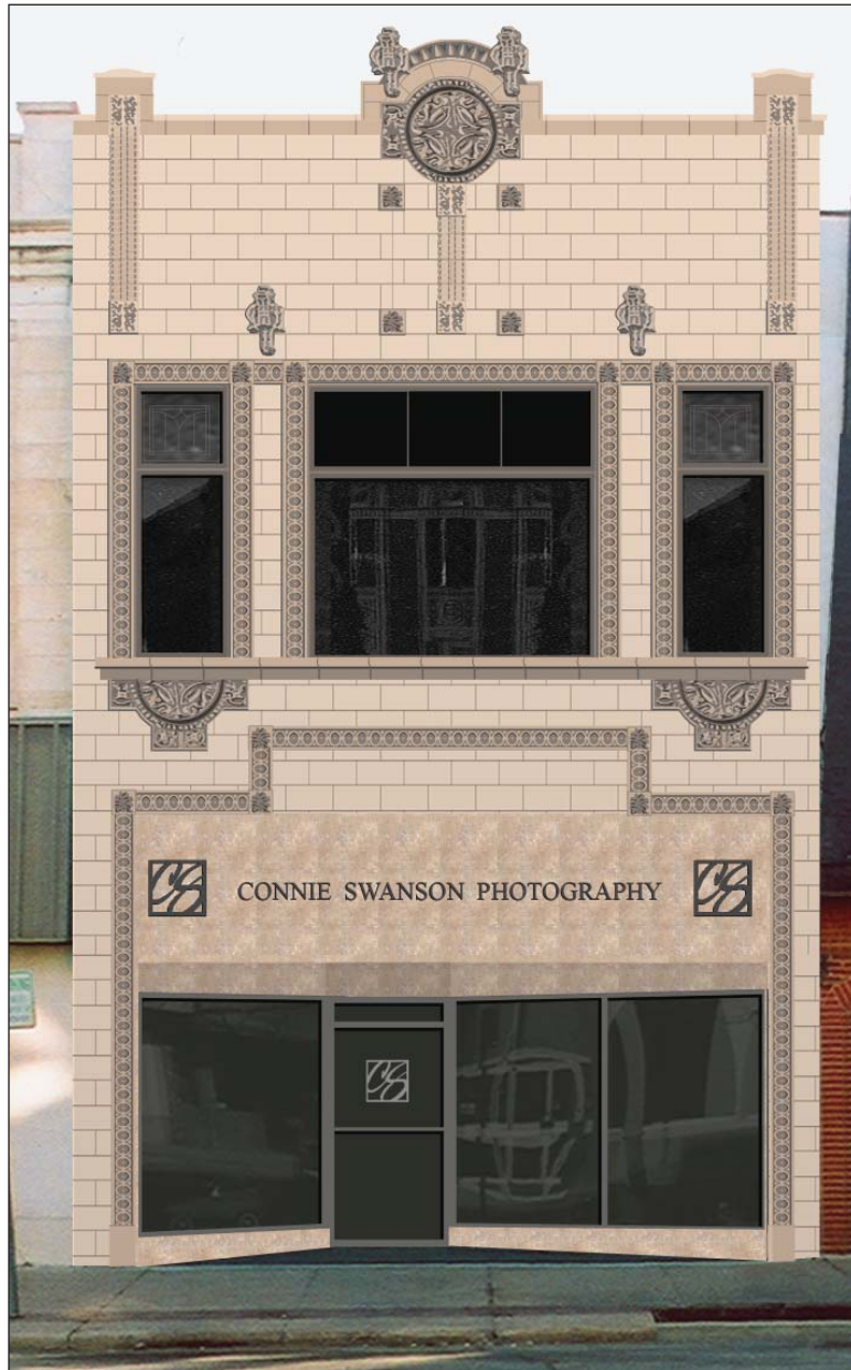
Image 21: Option 3. The former transom window and signboard opening has been replaced with porcelain tile, a sample of which is depicted in Image 17. The signage is flat cut metal in Times Roman font available from Gemini ( http://www.signletters.com ). The custom logo would be made using flat cut metal.
