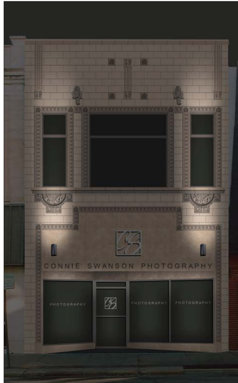
Image 19: Option 2. Cylinders' 300 LINE Enclosed Uplights are used to illuminate the building's terra-cotta details.
