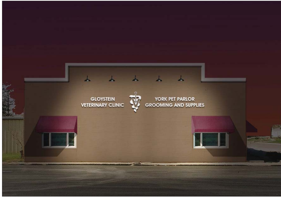
Image 7. Gooseneck Lamp. Five gooseneck barn-style lamps (see www.barnlightelectric.com ) mounted above the signage provide nighttime illumination on the east façade.
