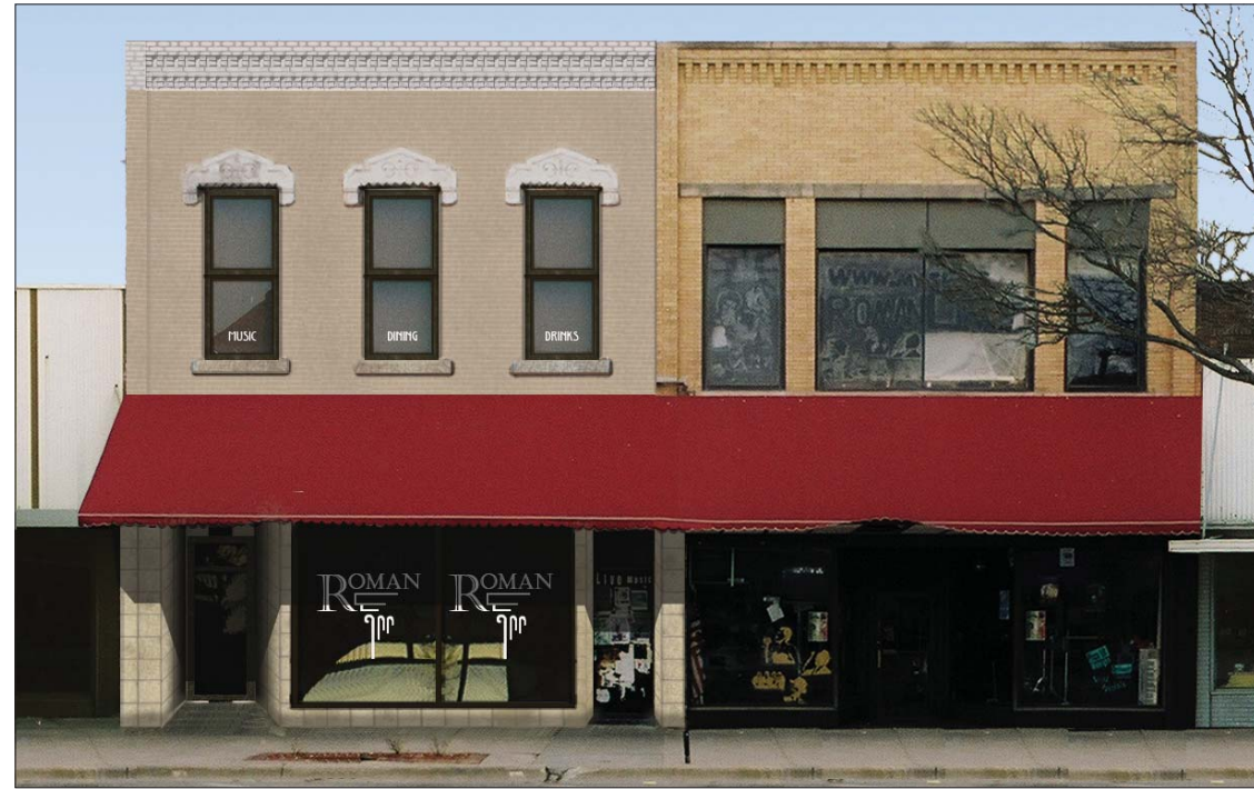
Image 9. Option 2.3: The brick on the second story of the Leach Building is repainted gray, similar to the existing color of the painted brick. One-foot-square yellow-gray porcelain tiles (Giove Levigato by Fiordo) are used for the exterior wall surfaces at the street level.
