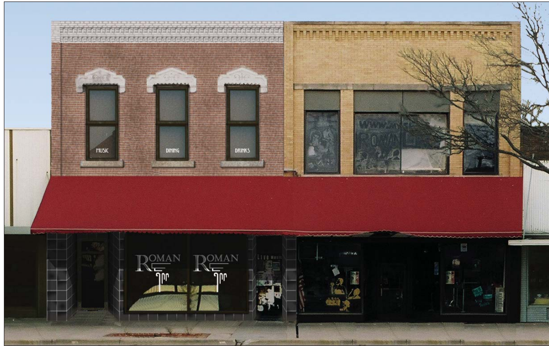
Image 8. Option 2.2: Paint on the brick of the second story of the Leach Building is removed to reveal the color of the original brick. One-foot-square black porcelain tiles (Ocean Cambrian Levigato by Fiordo) are used for the exterior wall surfaces at the street level.
