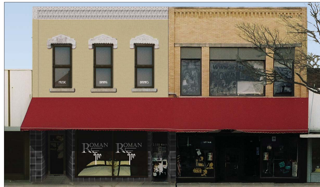
Image 7. Option 2.1: In the Option 2 series, the current storefront configuration in the Leach Building is retained, except that the wall is replaced with an anodized aluminum (bronze-colored) storefront with two adjacent storefront windows. Option 2.1 shows that the remaining exterior first floor wall surfaces on the Leach Building are covered with one-foot-square black porcelain tiles (Ocean Cambrian Levigato by Fiordo). The brick on the second story of the Leach Building is painted a yellow hue to match the unpainted second story brick on the adjacent building.
