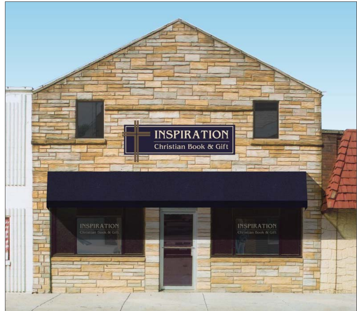
Image 9. Option 3 (East Facade): The awning is the same as described for Option 1 (Images 4, 5, and 7). The signboard is depicted in Image 11. The fonts for the vinyl lettering appliqué to the windows are the same as used for the signboard.
