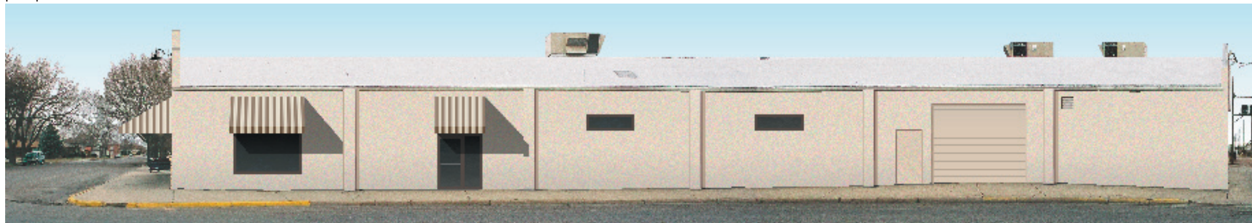
Image 6. Option 1 (East Facade): A new window has been added, as well as a new door with sidelight. A new steel door and overhead door are also shown to the right.
