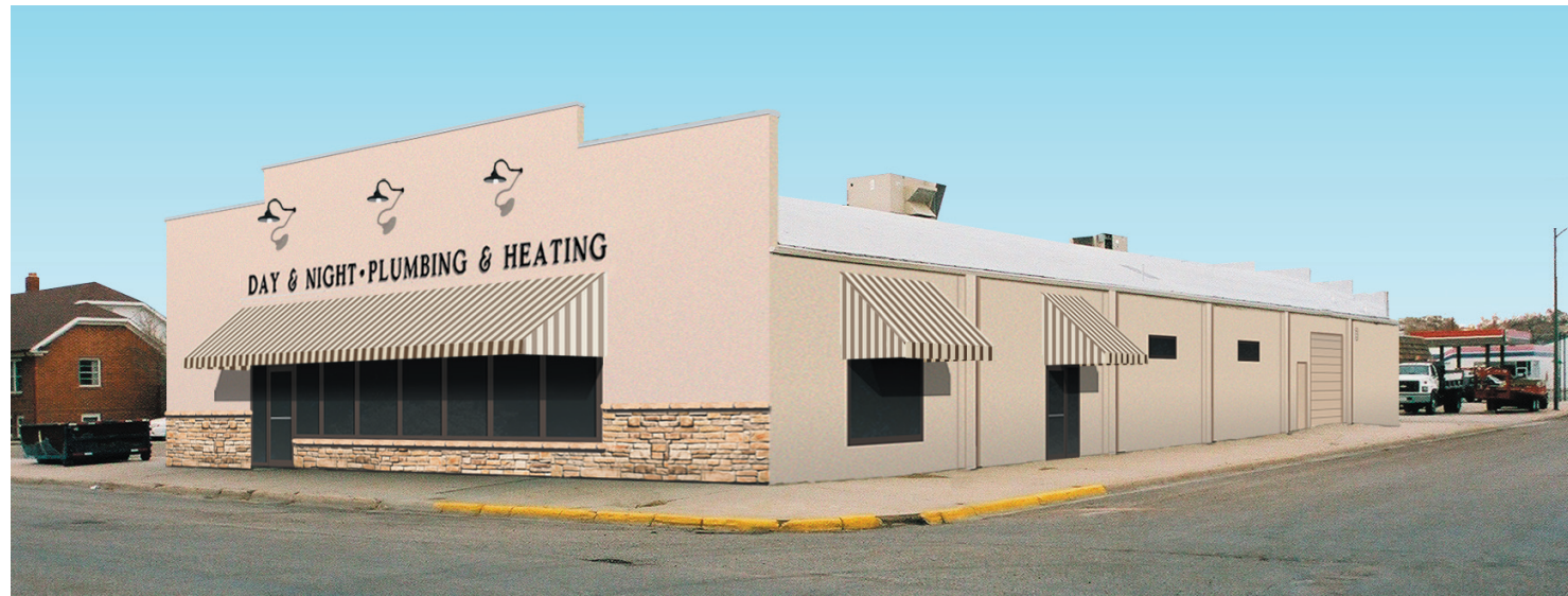
Image 4. Option 1 (Southeast Corner): The stucco or EIFS is similar in color to Pratt & Lambert's "Flagstaff" paint color (#2264). Similarly colored material on both facades gives the building further cohesion. New doors and windows with dark, bronze frames have been added to the building. Gooseneck downlighting is used to illuminate the signage and south-facing awning.
