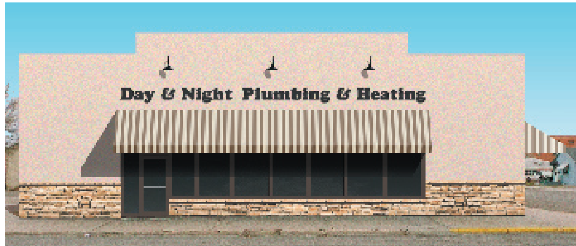
Image 29. Option 1 (South Facade, Alternative Signage): Dark gray (#333333), formed plastic, Cooper Black font available from Gemini.
