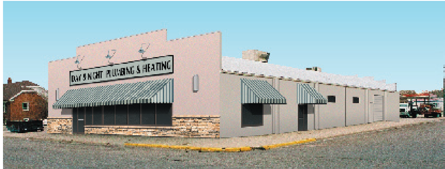
Image 24. Option 5 (Southeast Corner): The stucco or EIFS is similar in color to Pratt & Lambert's "Bristol Fog" paint color (#2281). Large, gooseneck downlighting is used to illuminate the signage and south-facing awning. Cylinder downlight fixtures bookend the south facade.
