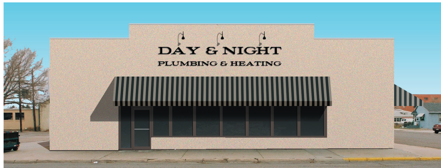
Image 10. Option 2 (South Facade): The signage on the storefront is black, formed plastic, Times Bold Extended font available from Gemini. Stucco or EIFS replace the metal on the south facade. Additionally, aluminum flashing has been added along the top of the parapet wall.
