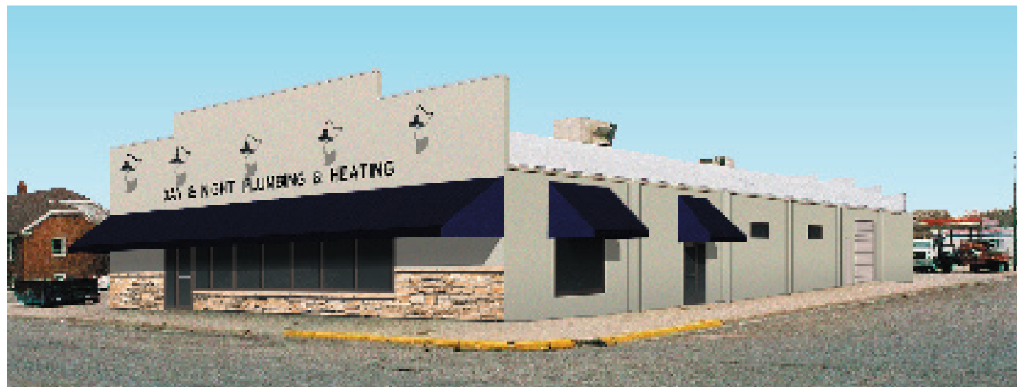
Image 19. Option 4 (Southeast Corner): The stucco or EIFS is similar in color to Pratt & Lambert's "Pebble" paint color (#2282). Large gooseneck downlighting is used to illuminate the signage and south-facing awning. This awning runs the entire length of the facade.
