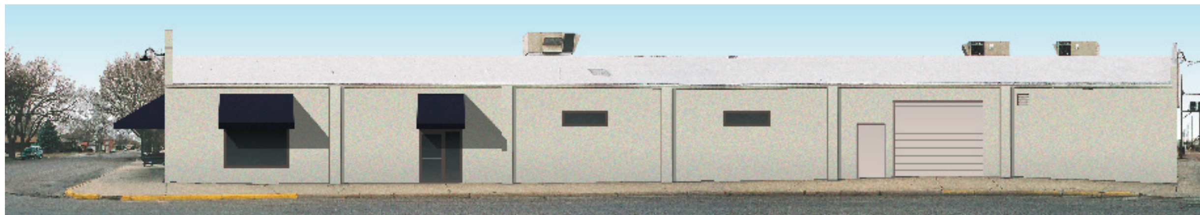
Image 16. Option 3 (East Facade): A new window has been added, as well as a new door with sidelight. A new steel door and overhead door are also shown to the right.
