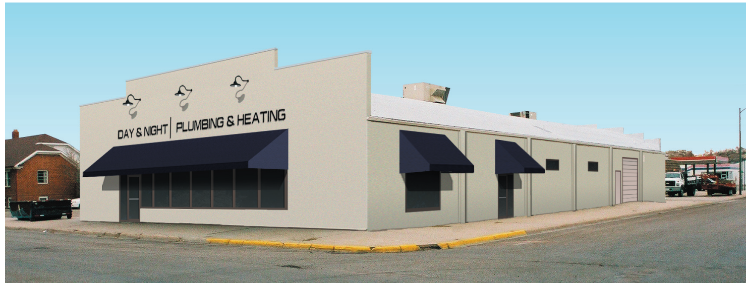
Image 14. Option 3 (Southeast Corner): The stucco or EIFS is similar in color to Pratt & Lambert's "Pebble" paint color (#2282). Gooseneck downlighting is used to illuminate the signage and south-facing awning.
