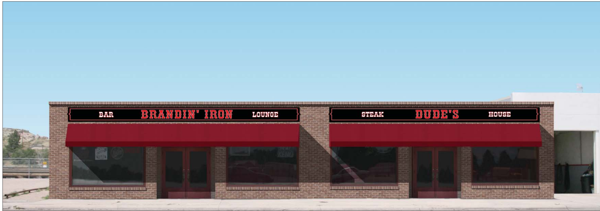
Image 9. Option 4 (South Facade): This option depicts new signage. In part, this is in case there is extensive damage to the material behind the canopy, and the new signs can be used to conceal the damage. The two large signs mounted on the roof of the building have been removed and signboards have been placed above each awning. The signboards use "Thunderbird " and "OldTowne536D" fonts. The awning fabric depicted is "Jockey Red" #4603 by Sunbrella.
